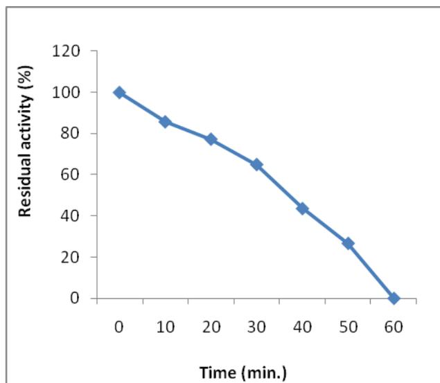
**Figure 3: Thermal stability of free phytase at 65°C**
